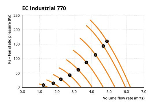
Aerodynamic performance is measured in accordance with ISO 5801 (Type A installation) in our AMCAaccredited laboratory.
