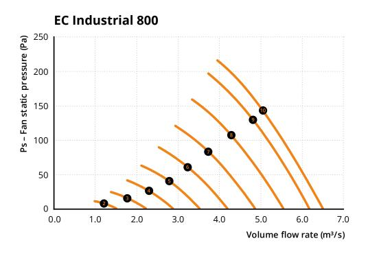
Aerodynamic performance is measured in accordance with ISO 5801 (Type A installation) in our AMCA-accredited laboratory.
