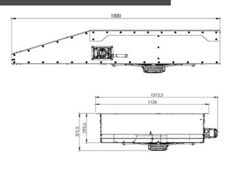
Approximate Fan Weight: 165 KG All dimensions are in mm.
